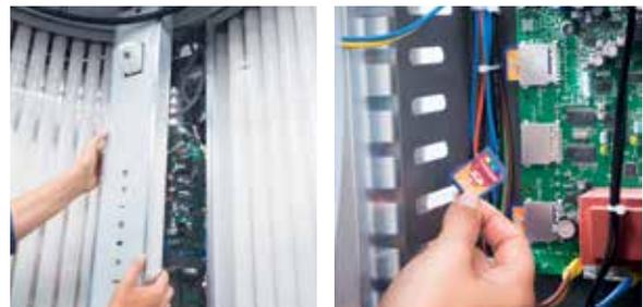
By removing the Ambient FlowLight panel inside the V<sub>8</sub> you have access to all electronic components.
